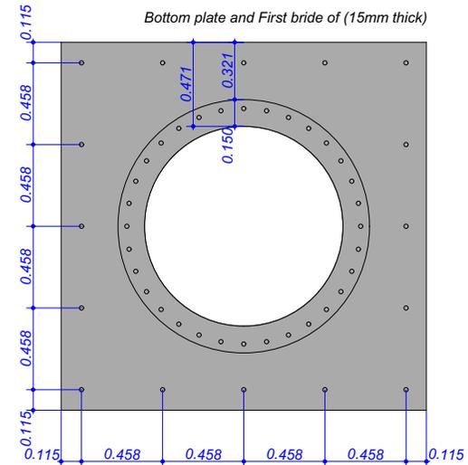
STRUCTURAL DETAILS FOR SMOKE CHIMNEY
